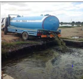
Plate 11-6: Waste water discharged at waste stabilization ponds in Dodoma and Dar es Salaam Cities
